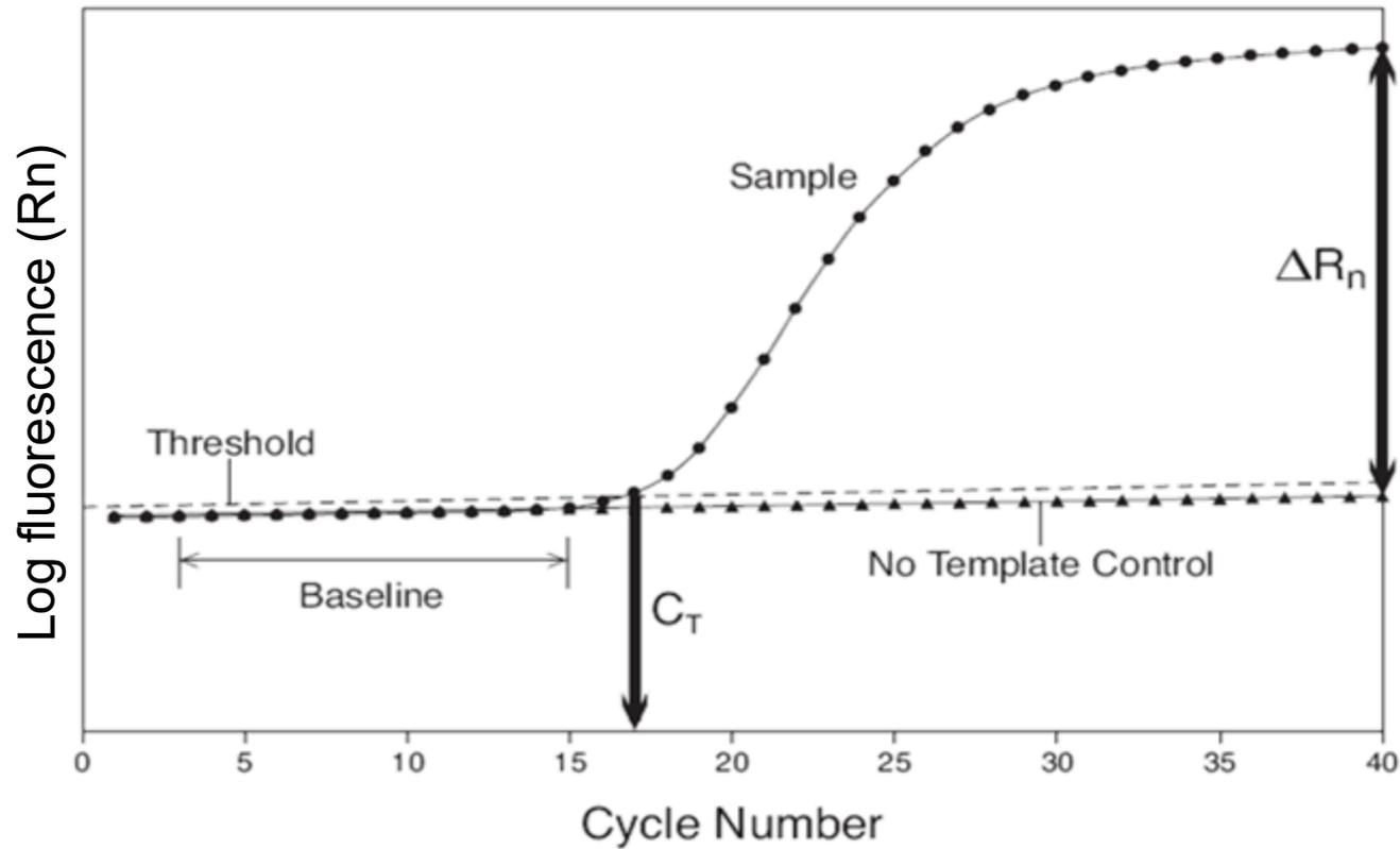
**Baseline** - The baseline phase contains all the amplification that is below the level of detection of the real time instrument.
