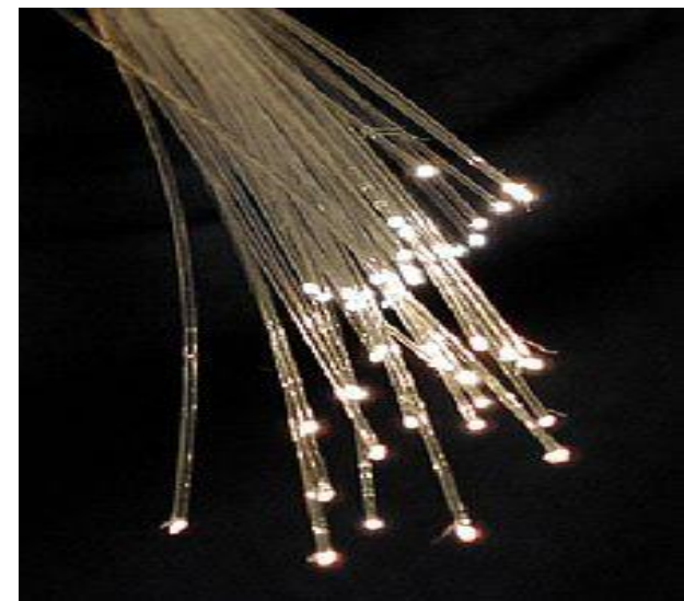
Bundle of optical fibers composed of high purity silica.
