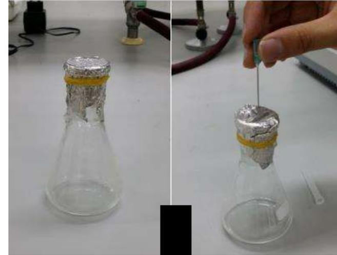
1 جهزنا الأدوات ووزناهم + We made a holes n Al foil to allow to liquid to evaporate
