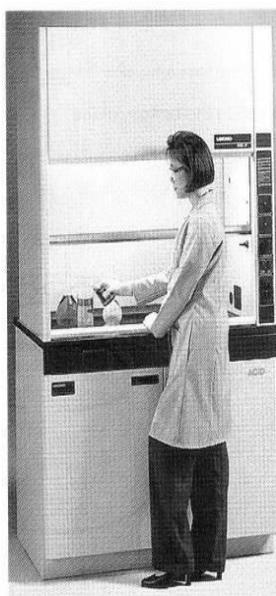
**Figure T.12a** A modern laboratory fume hood.
