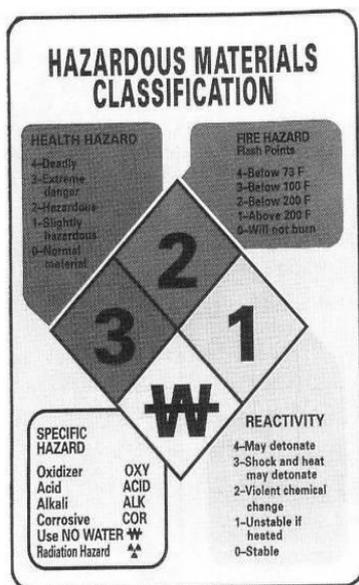
**Figure T.3b** Hazardous materials classification system.
