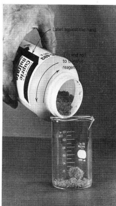
**Figure T.9b** Tilt and roll the reagent bottle back and forth until the desired amount of solid chemical has been dispensed.
