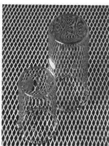
**Figure T.2a** Invert clean glassware on a paper towel or rubber mat to air-dry.
