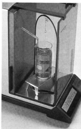
**Figure T.6d** Electronic analytical balance, sensitivity of  $\pm 0.00001$  g.
