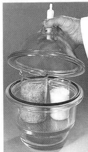
**Figure T.15b** A simple laboratory desiccator (left) or a glass desiccator (right) contains a desiccant (usually anhydrous  $\text{CaCl}_2$ ) to provide a dry atmosphere.
