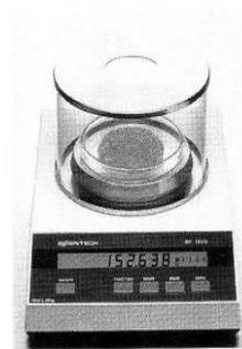
**Figure T.6b** Electronic top-loading balance, sensitivity of  $\pm 0.01$  g and/or  $\pm 0.001$  g.
