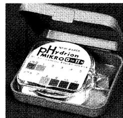
**Figure 6.6** The pH of a solution can be estimated with pH paper, a strip of paper that is impregnated with a mixture of acid-base indicators. A gradation of colors on the pH paper approximates the pH of the solution.
