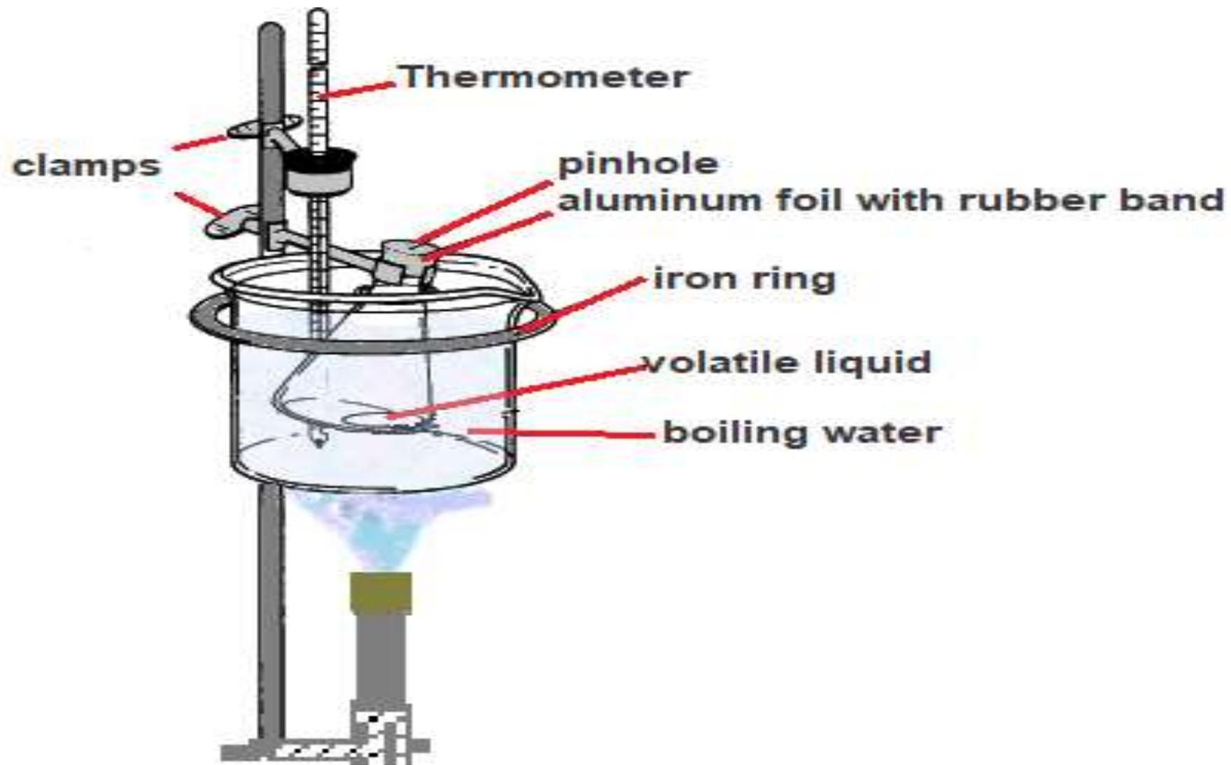
Apparatus for determining the molar mass of a volatile liquid.
