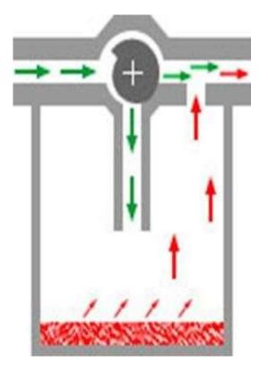
The purpose of an anaesthetic vaporiser is to produce a controlled and predictable concentration of anaesthetic vapour in the carrier gas passing through the vaporiser.
