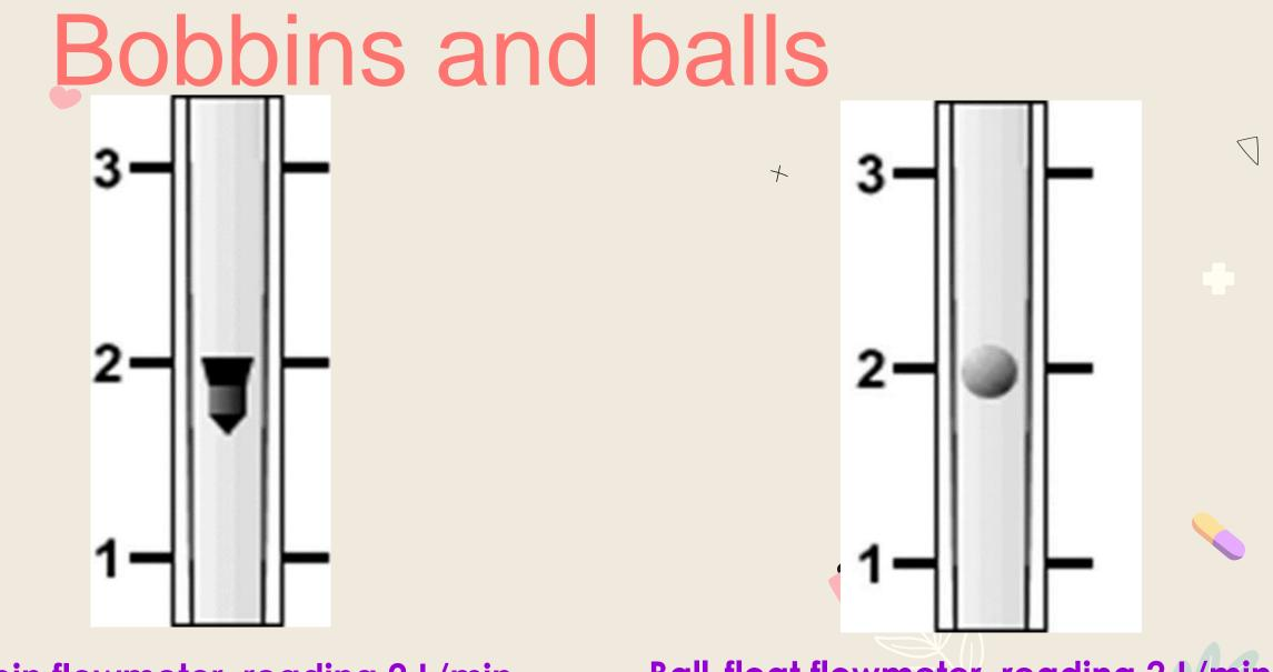
**Bobbin flowmeter, reading 2 L/min**
