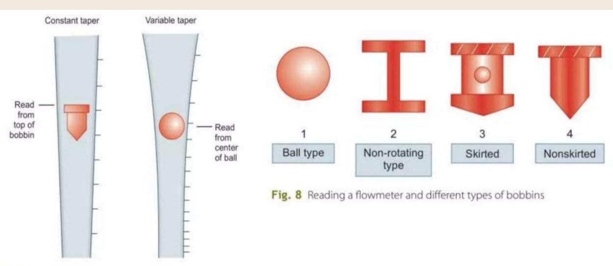
Fig. 7 Rotameters with bobbins
