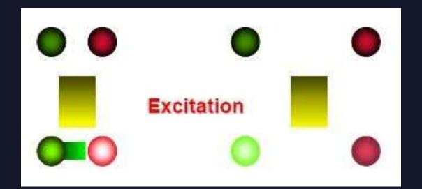
The 5' nuclease active polymerase starts to degrade the probes, separating the dyes from the quenchers. While the polymerase continues its elongation, the reporter dyes and quenchers are drifting apart, leaving the quenchers unable to absorb fluorescence emitted from the dyes. The result is a detectable fluorescence signal from the sample.
