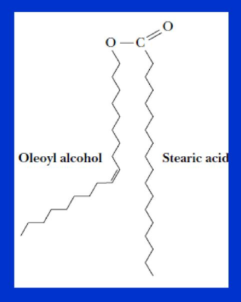
An example of a wax: Oleoyl alcohol is esterified to stearic acid in this case
