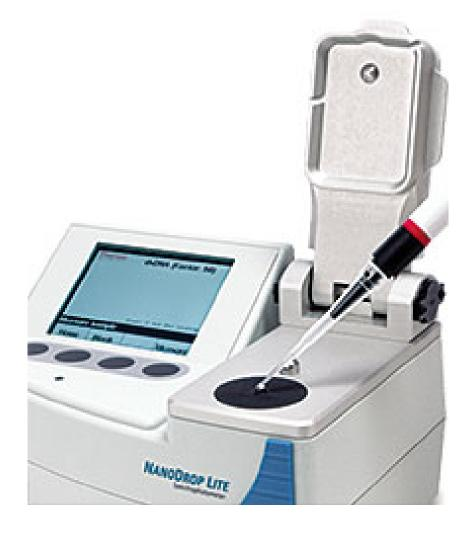
NanoDrop is automatically calculate the concentration in ng/ $\mu l$
