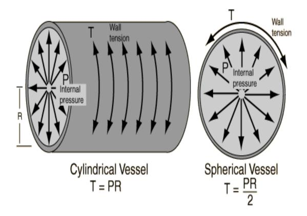
\*The tension in cylindrical vessel is higher (pressure and radius are higher) than spherical vessel.
